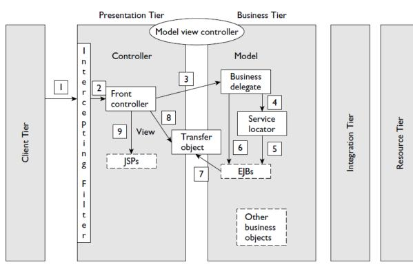
a. A request is trapped by an Intercepting Filter (1)—if the filter allows it, the request passes on to a Front Controller (2). The Front Controller makes use of a Business Delegate to obtain business data (3). The Business Delegate uses a Service Locator (4) to find the business component it needs (5)— often an EJB. The Business Delegate requests data (6), which it gets back in the form of a Transfer Object (7), and returns this to the Front Controller. The Front Controller
